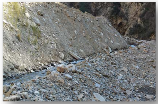
Designated overburdens site blocking the natural waterways of the stream at Damchulum stone quarry
