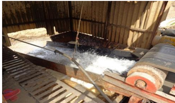
(Cleaning of raw mineral sand)
