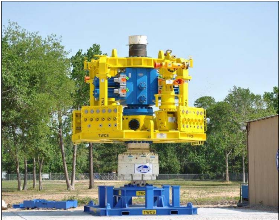
Figure 3: A Capping Stack Ready for Deployment
